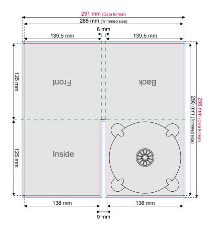
3 mm trimming edgeTrimmed sizePerforation line / grooving
