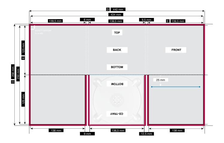
3 mm trimming edgeTrimmed sizePerforation line / grooving
